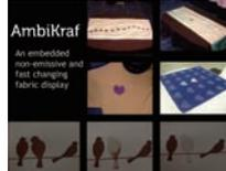
AmbiKraf は novel non-emissive analog fabric display that has rapid color changing capability based on embedded semiconductor Peltier junctions that are integrated with the soft fabric, enabling novel animations and interactive scenarios in the normal daily fabrics.
